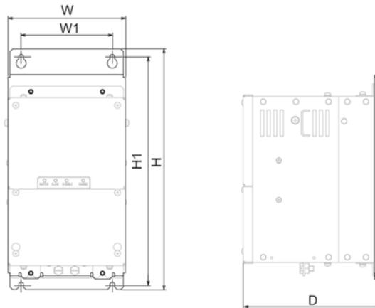
**Figure 18: Retrofit Attachment for CDBR-2110D, CDBR-4220D, CDBR-5110D, and CDBR-5300D**
