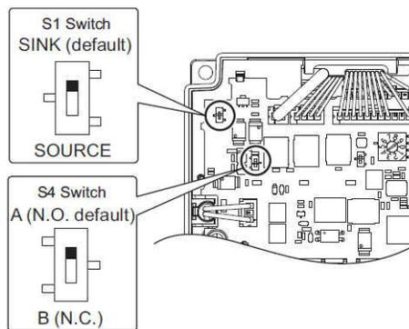
**Figure 13: Setting Sink/Source Switch (S1) and N.O./N.C. Switch (S4)**
