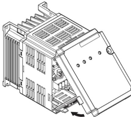
**Figure 6: Reattach the Front Cover**
