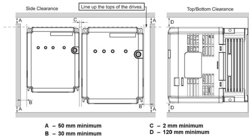
**Figure 2: Space Between CDBR braking units (Side-by-Side Mounting)**
