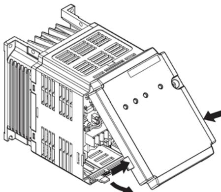
**Figure 4: Push the Tabs Inward and Pull Forward on the Front Cover**
