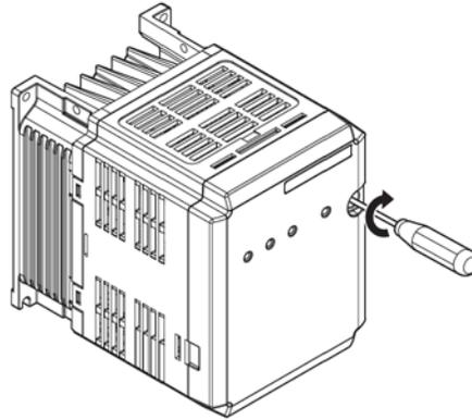
**Figure 7: Tighten the Front Cover Screw**
