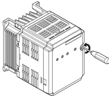
**Figure 3: Loosen the Screw Securing the Front Cover**
