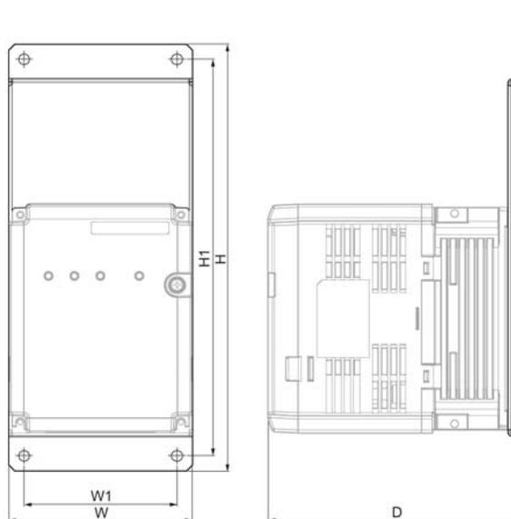
**Figure 16: Retrofit Attachment for CDBR-5037D**
