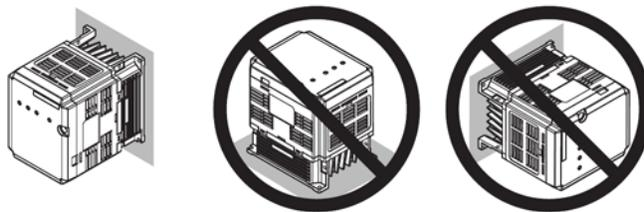
**Figure 1: Correct Installation Orientation (Braking Unit)**
