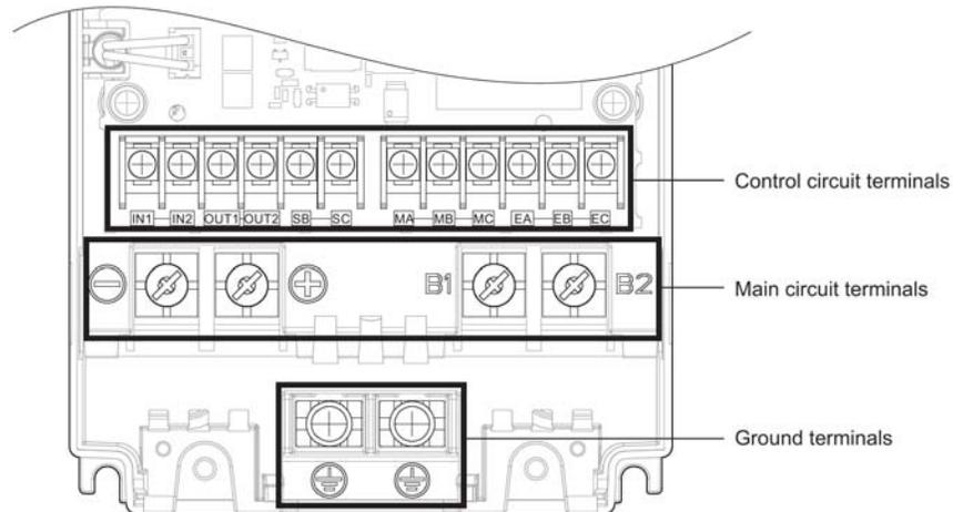
**Figure 5: Wiring the Terminals**
