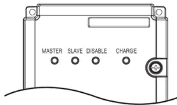
**Figure 8: CDBR Braking Unit LED Display**
